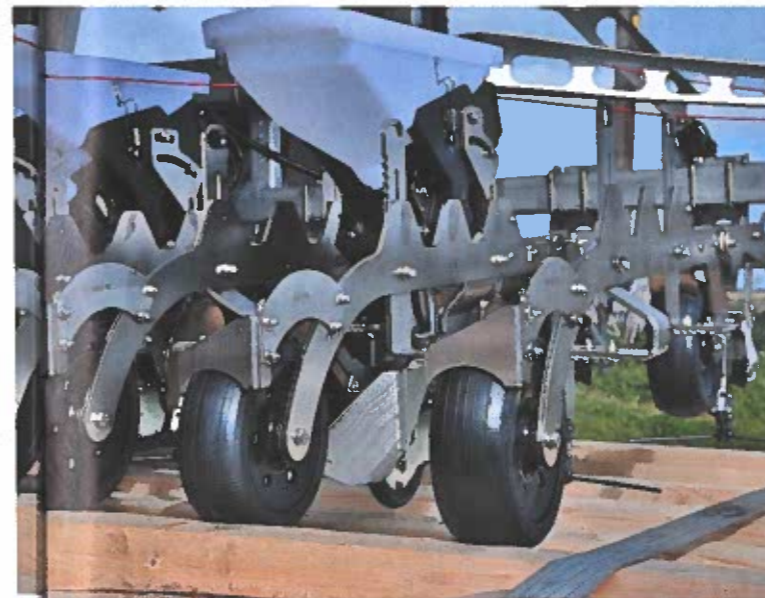
Above: Trawling arms are mounted on a toolbar at the front of the machine. All parts are made from laser-cut stainless steel
