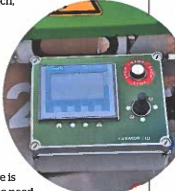
Above: The FD20 is equipped with an operator control box for set-up and manual operation. It requires an RTK base to operate but one base will operate multiple machines
