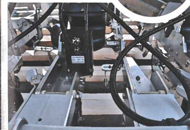
Left: The FarmDroid uses two trailing arms or trawlers (active and passive) for each row. The powered active trailer is used for seeding and inter-plant hoeing. The passive arm is for inter-row tools only
