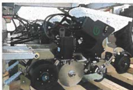
The seeding unit on the active trailer (left), is tilted out of the way when weeding (centre). A knife mounted on an electric actuator (right) carries out the intra-row weeding.
