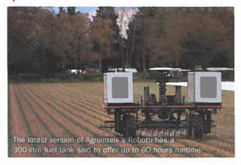
The Robotti LR 'long range' has its three-point linkage lift capacity increased to 1,250kg and a new GPS tower at the centre of its frame. Navigation is via RTK GPS with 3D LIDAR scanners offering obstacle detection.
